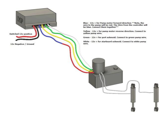
Manual switch control. This can be added to use the mechanical buttons that likely came with your trim tabs. Disconnect all wires from the switches and only connect them to the controller as shown. If you fail to wire this correctly, it can permanently disable the Controller.
